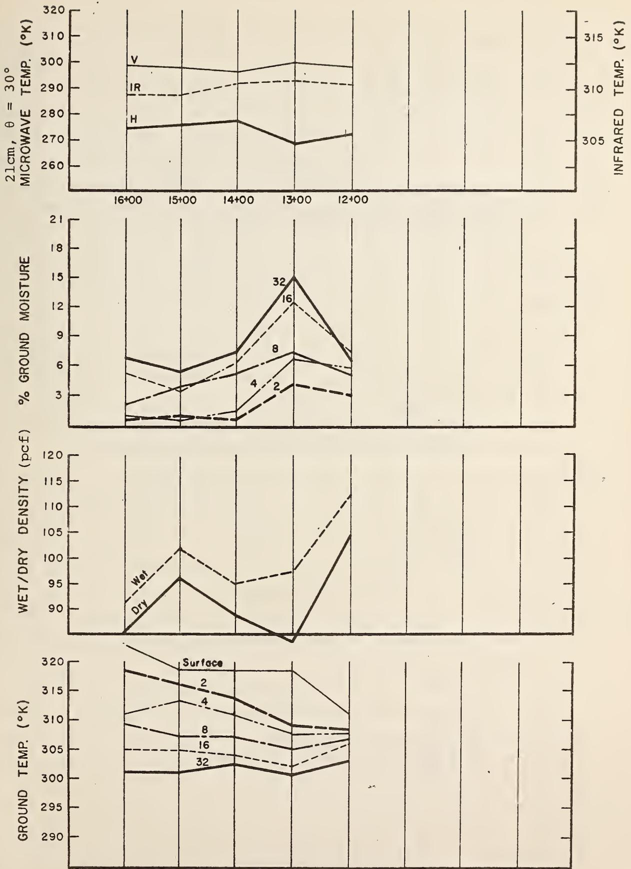
Figure 3.13 Correlation of Measurements Galena Line A, Run 1
